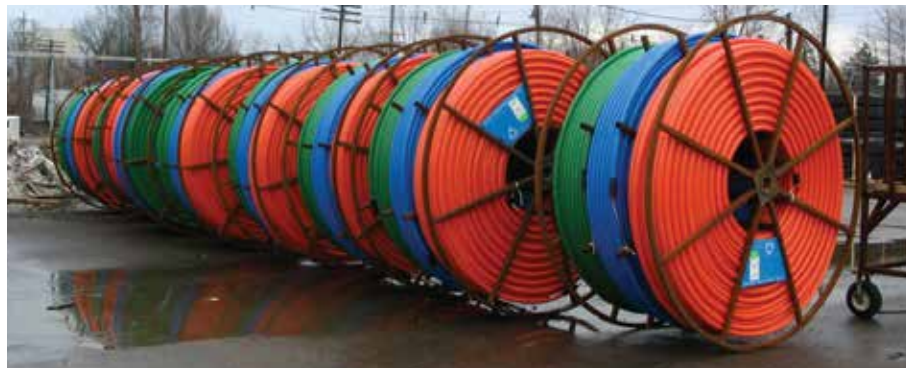
Divided Reels with 3 conduits on one reel.
