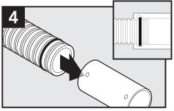
Insert the gasketed end of the conduit into coupler. The lock ring on the inside surface of the coupler should snap into a matching corrugation. A light coating of water-based lubricant should be used to aid in installation.
