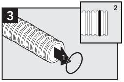
Take one duct and install O-ring gasket. The interior of the O-ring has a high profile that snaps into place. Ensure it is seated in the second corrugation.
