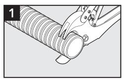
Ensure your conduit has a clean, perpendicular cut. Cut the duct in the valley of the corrugation to ensure proper alignment.
